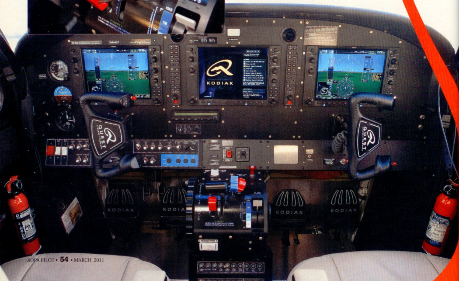
Like the rest of the Kodiak, the cockpit is sturdy and durable. The power pedestal (left) controls the PT6, and synthetic vision is standard on the G1000.
