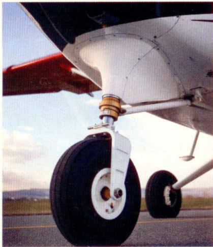
Unfaired flap tracks (top) and oversized tires (above) show that Kodiak designers value simplicity and strength more than speed. The big door (top right) is large enough for cargo on pallets.
